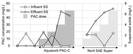
Figure 6. Changes in suspended solids during the PAC trial runs with the pile cloth filter. SS values below detection limit are shown as zero.
