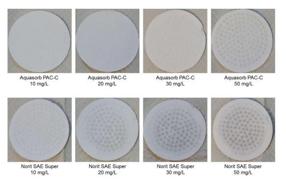
Figure 10. Comparison of the results of filtration tests for the Minifilter effluent with different doses of AquaSorb® PAC-C and Norit SAE Super carbons.
