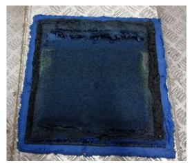
Figure 11. Pile cloth filter after the end of piloting with PAC, after thorough washing with water.
