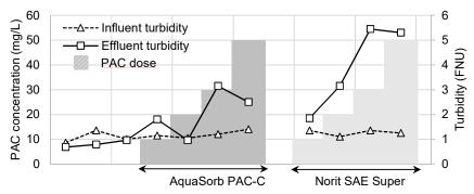
Figure 5. Changes in turbidity during the PAC trial runs with the pile cloth filter.
