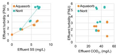
Figure 8. Correlation between effluent turbidity and suspended solids.
