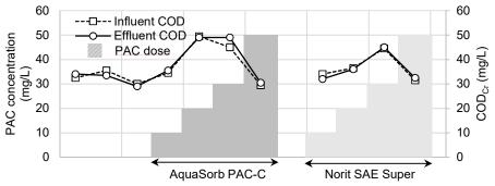
Figure 7. Changes in COD during the PAC trial runs with the pile cloth filter.
